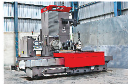
Horizontal Boring & Milling machine with boring facing head.
